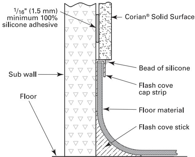
**FIGURE J-4: Wall Base Detail With Dado And Flash Cover**
