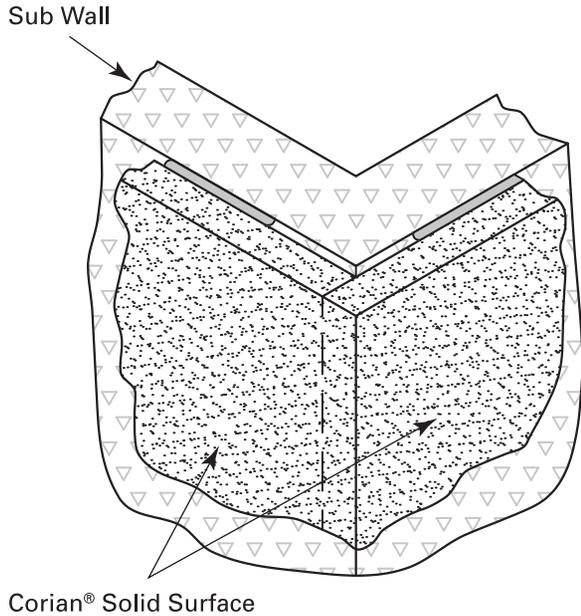
FIGURE C-2: Alternative Outside Corners – Silicone Seam
