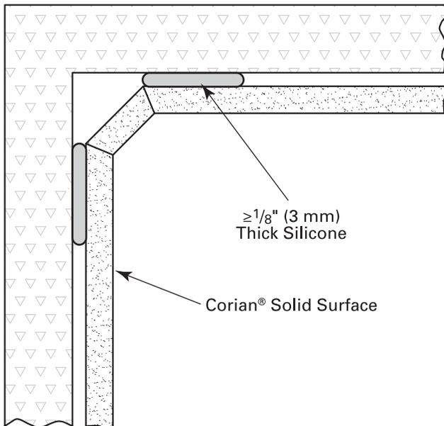
FIGURE E-2: Hard Seamed Corners – Thermoformed Cove
