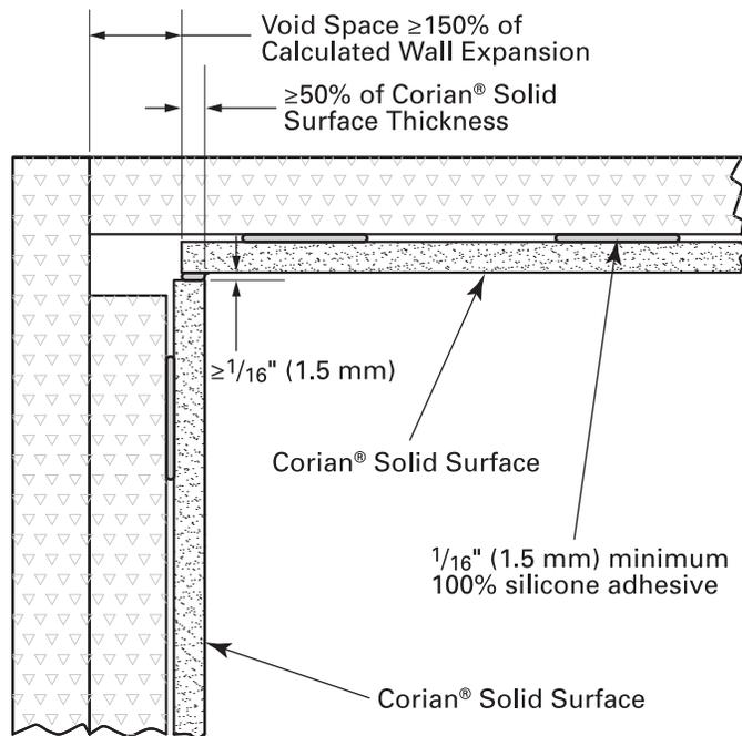
TABLE 5: SUGGESTED VOID SPACE AS FUNCTION OF EXPECTED TEMPERATURE CHANGE FOR LAPPED CORNER WITH EXPANSION SPACE (REFERENCE FIGURE F-1)
