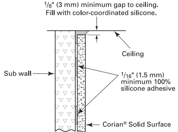
**FIGURE K-2: WALL CEILING DETAIL WITH TRIM**
