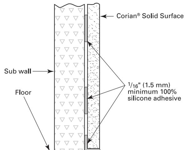
**FIGURE J-2: Wall Base Detail With Trim**
