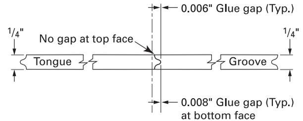
**CAUTION:** Demonstrate tongue and groove or wavy edge seaming is acceptable for the Corian® Solid Surface color chosen. Several Corian® colors are quite translucent, e.g., Cameo White, and unacceptable seam shadows can be apparent when these alternative edge geometries, e.g., tongue and groove, are used. Also be sure to clean all seaming edge surfaces before applying joint adhesive to keep visible dirt lines out of the seams.
