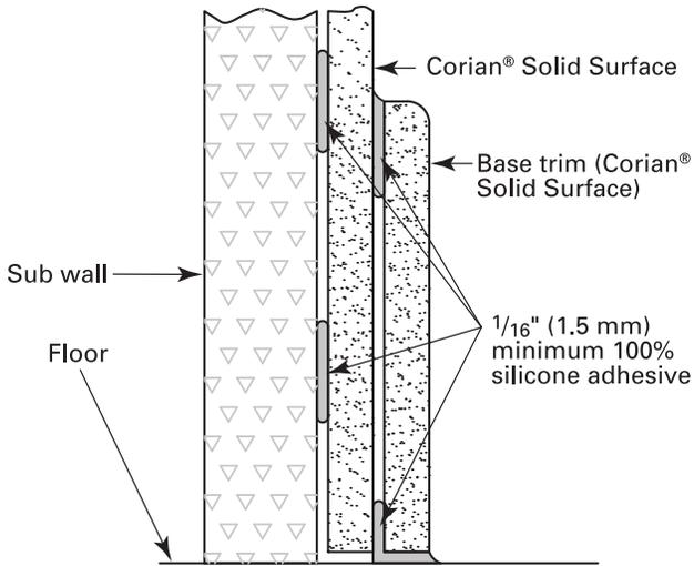
**FIGURE J-3: Wall Base Detail With Flash Cover**
